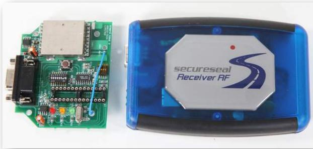
**DoorRF** is a wireless door sensor that transmits an alert or data packet when the door is opened or closed. This can provide reliable access data that can be linked to telematics for unauthorised GPS linked events.
